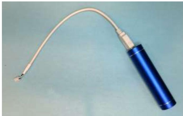
Both of the above power supplies can plug into the AUX POWER (2 pin JST-PH) connector on the Kookaberry given the appropriate cable connectors.
